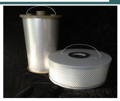
Jaxon's *Trans-Dri* filter element is designed to remove free and dissolved water from insulating oils. Moisture can be lowered to less than 10 PPM without the use of heat and vacuum processing.
